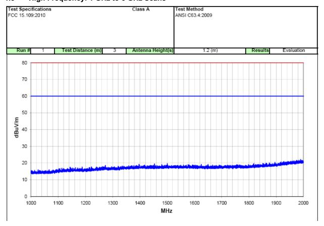
Figure 1.2: HF Scan Class A Test Results
