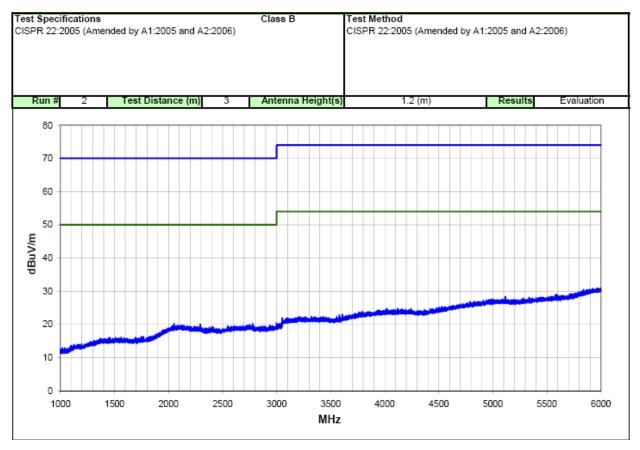
Figure 1.3: HF Scan Class B Test Results
