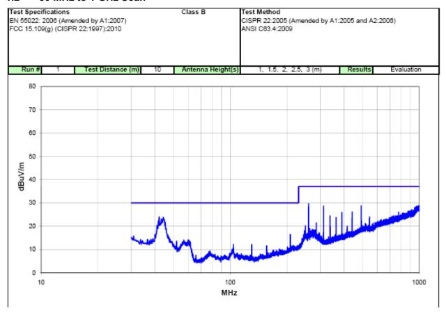
Figure 1.1: RE Scan Class B Test Results—Evaluation
