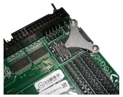
Figure 6.2: Torpedo SOM Hold-Down Clip
