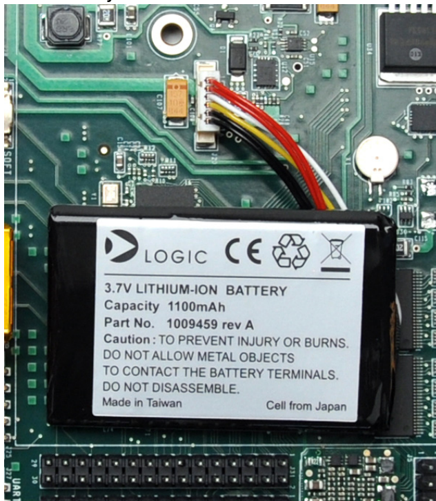
Figure 2.4 – Connect Battery to Baseboard
