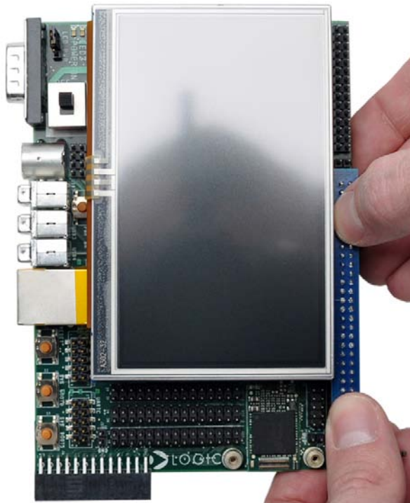
Figure 2.5 – Connect LCD to Baseboard
