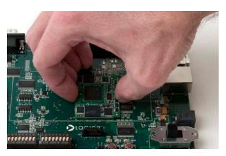
3. To connect the AM1808 SOM-M1, align the SOM over the three board-to-board connectors. Using even pressure, press straight down over the connectors to mate boards. Visually verify that all three connectors have fully mated.
