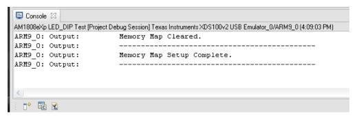
To run the program, select Target > Run from the menu bar. (NOTE: If you receive a message stating "Error during: Execution, Initialization, Control," click Cancel, select Target > Terminate All from the menu bar, press the reset button on the baseboard, and repeat steps 7-9.)
