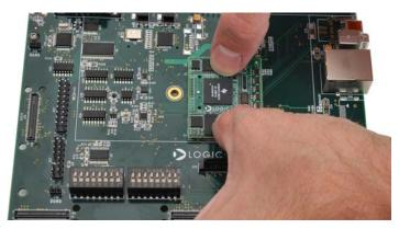
4. Connect the 4.3" LCD by inserting into the baseboard LCD connector and pushing down over the connector until the LCD ejector levers move to a vertical position. **CAUTION:** The solder points on the LCD connector PCB may be sharp; use caution when connecting the LCD.
