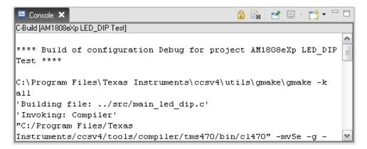
Once the Console window prints the message "Build Complete," select Target > Debug Active Project from the menu bar. (NOTE: If you receive a message stating "Error connecting to the target," press the reset button on the baseboard and then click Retry.)
