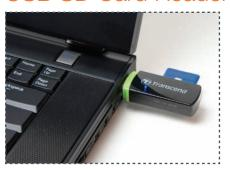
To prepare your workstation for software development, power off the kit, remove the SD card and insert into the included USB SD card reader. Connect the SD card reader to your host PC.
