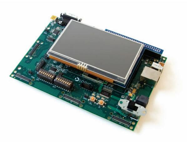
Congratulations on your purchase of the Zoom AM1808 eXperimenter Kit. This Zoom Development Kit provides a product-ready hardware and software platform for evaluating the functionality of the Texas Instruments (TI) AM1808 processor and the Logic PD System on Module (SOM).
