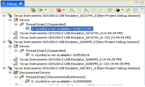
Figure 2.3: Selecting the DSP Core
