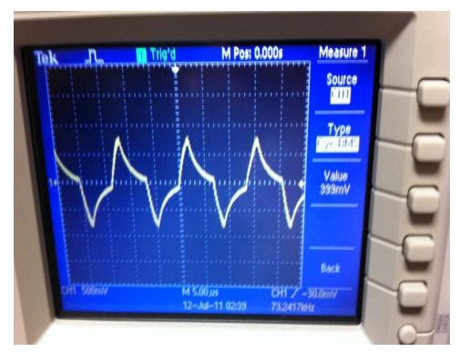
Figure 3.5: UPP Test ADC in Samples Collected and Displayed with the Oscilloscope Image
