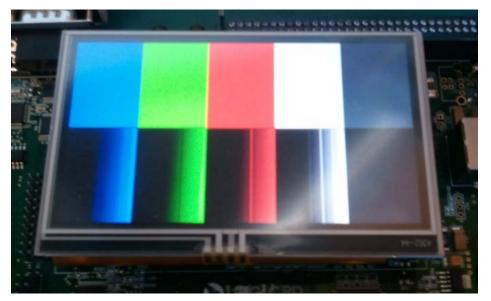
Figure 3.1: Graphics LCD Test Image
