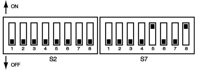
Figure 2.2: S2 & S7 DIP Switch Required Settings
