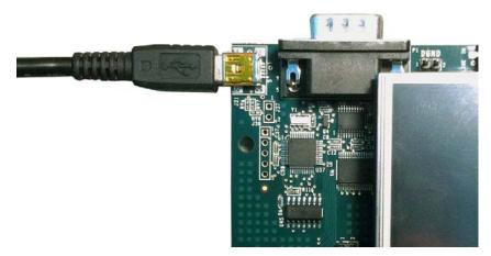
Figure 2.1: Connection to Emulation USB Port
