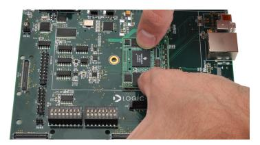
5. Connect the 4.3" LCD by inserting into the baseboard LCD connector and pushing down over the connector until the LCD ejector levers move to a vertical position. **CAUTION:** The solder points on the LCD connector PCB may be sharp; use caution when connecting the LCD.
