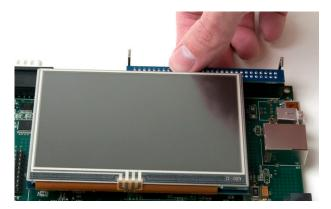
6. Place the OMAP-L138 SOM-M1 into the ESD protective bag that was used for the TMS320C6748 SOM-M1. Keep with EVM components for future use.
