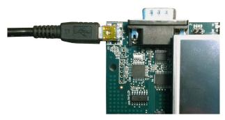
As soon as the USB cable connects to your host PC, Windows should automatically recognize that new hardware has been connected and install the necessary drivers. Power on your OMAP-L138 EVM and continue with the next section.
