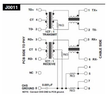
Figure 2.1: Example Magnetics Design, Pulse J0011
