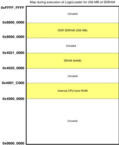
Figure 1.1: DM3730/AM3703 Torpedo + Wireless SOM Hardware Memory Map
