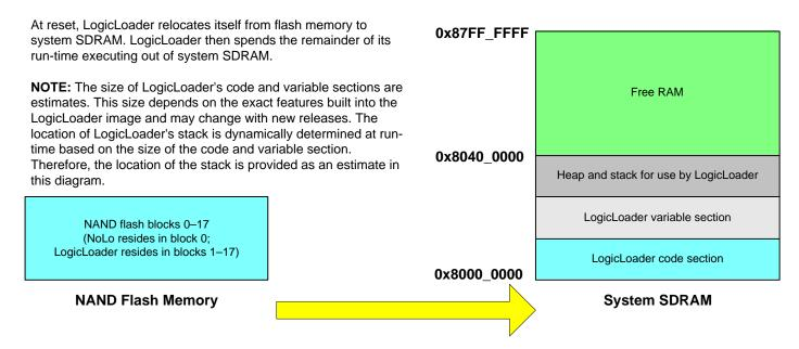
Figure 1.3: LogicLoader RAM Execution Environment
