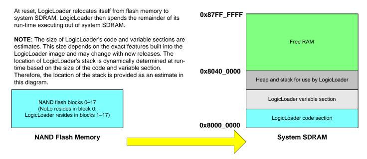
Figure 1.3: LogicLoader RAM Execution Environment
