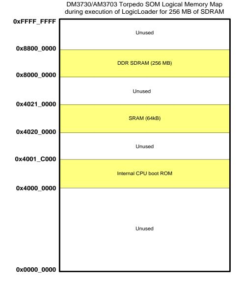
Figure 1.1: DM3730/AM3703 Torpedo SOM Hardware Memory Map
