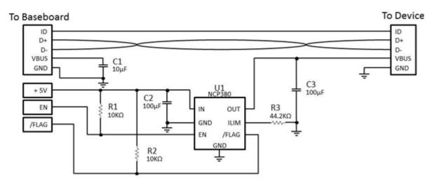
Figure 1 Example Using NCP380
