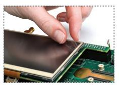
Before using LCD touch screen, remove protective plastic film covering.
