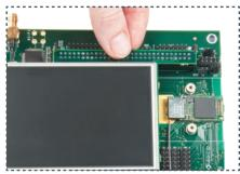
Press straight down on LCD board until connector levers move to vertical position.
