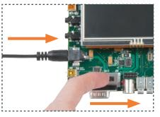
Connect power to baseboard and electric outlet; switch power on.
