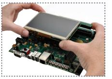
Align keyed connector on LCD board with baseboard 60-pin LCD connector.
