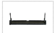
Locate 60-pin LCD connector on baseboard (SOM-LV: J11, Torpedo: J3).
