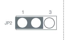
If connecting to Torpedo baseboard, place jumper JP2 across pins 1 and 2.
