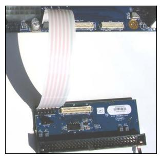
Figure 2 — Connect 6-pin ribbon cable
