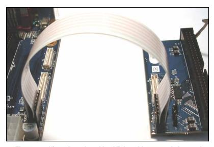
Figure 3 — View of touch and backlight cables properly inserted
