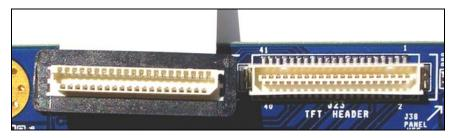
Figure 4.1 — Keyed connectors only fit in one direction
