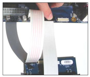
Figure 4.2 — Connect the TFT ribbon cable
