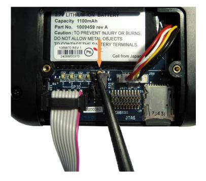
2. Plug a 5V source onto the MDK J58.1 jumper pin. **Note:** The PCB silkscreen label pointing to J58 is located under the battery. In the picture below, J58 pin 1 is the left pin.
