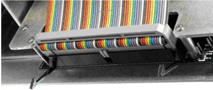
Figure 3.7 – Connect Ribbon Cable to the Display Kit
