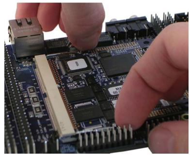
Figure 6 - Release SODIMM Connector Locks
