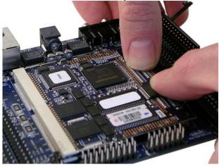
Figure 3 – Apply Equal Pressure Directly above Expansion Connectors
