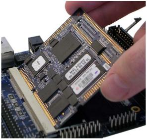
Figure 2 – Insert Card Engine into SODIMM Connector
