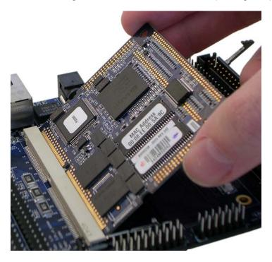
Figure 7 – Remove Card Engine from SODIMM Connector
