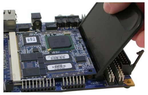
Figure 5 – Use Tool to Extract Card Engine
