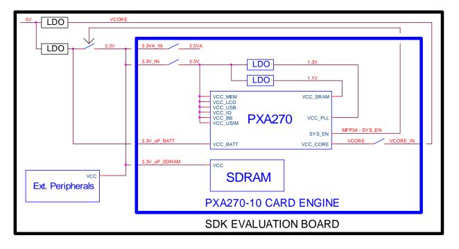
Figure 3.1: SDK Power Supply Implementation
