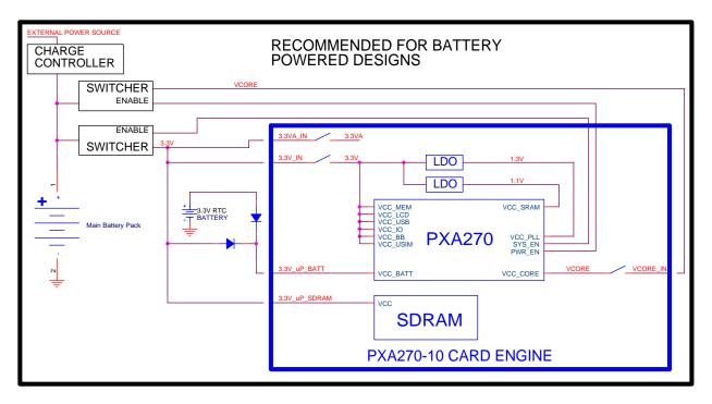
Figure 3.3: Using PWR\_EN and SYS\_EN to Control Switching Regulator
