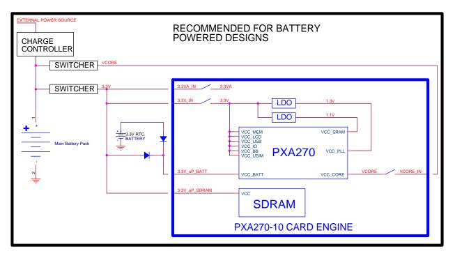
Figure 3.2: Typical Block Diagram for Battery Powered Device
