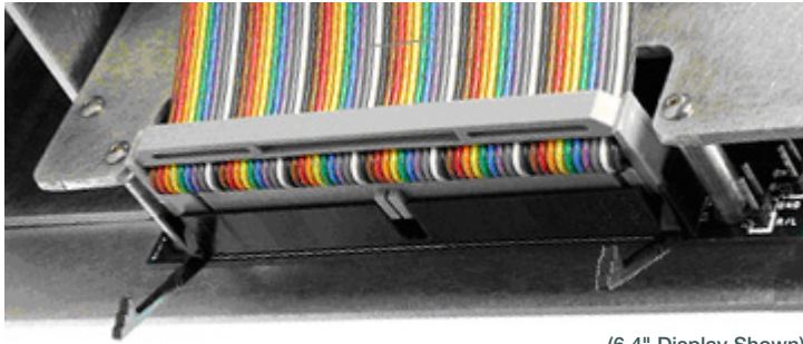
Figure 3.6 – Connect Ribbon Cable to the Display Kit
