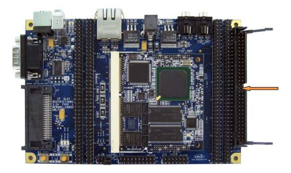
Figure 2.1: 60-pin LCD Connector on the Zoom SDK Baseboard
