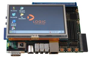
WINDOWS EMBEDDED CE 6.0 BSP RUNNING ON AN OMAP35X TORPEDO DEVELOPMENT KIT
