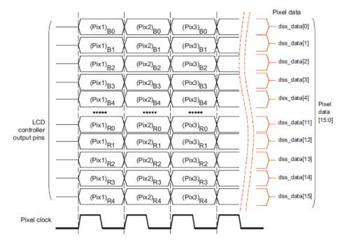
Figure 3.5: CPU 16-bit LCD Output and Data Format for Parallel Interface
