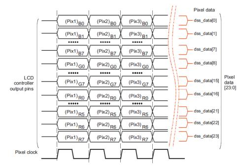
Figure 3.6: CPU 24-bit LCD Output and Data Format for Parallel Interface
