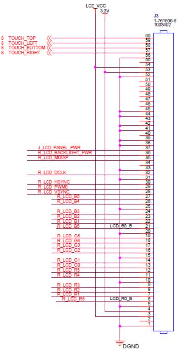
Figure 3.2: Torpedo Launcher Baseboard J3 60-pin 0.100" Header Pinout
