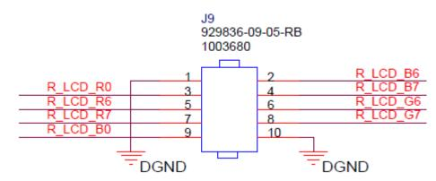
Figure 3.3: SDK2 Baseboard J9 10-pin 0.100" Header Pinout
