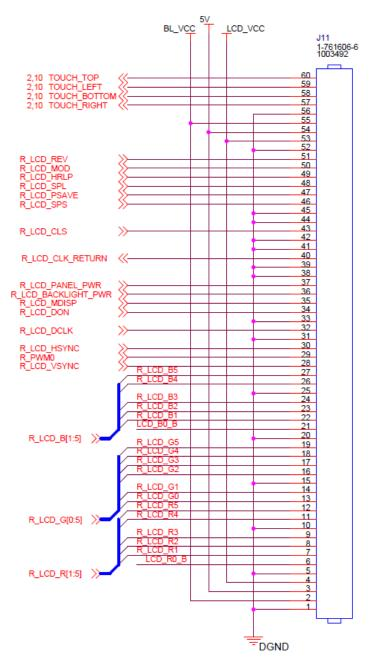
Figure 3.1: SDK2 Baseboard J11 60-pin 0.100" Header Pinout
