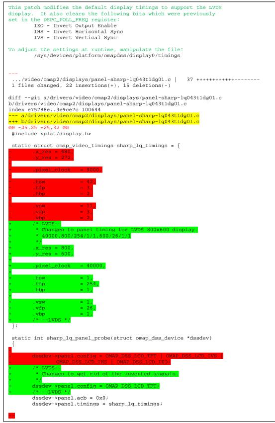
Figure 7.2: Panel-sharp-lq043t1dg01.c Patch
