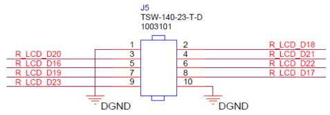
Figure 3.4: Torpedo Launcher 3 J5 10-pin 0.100" Header Pinout
