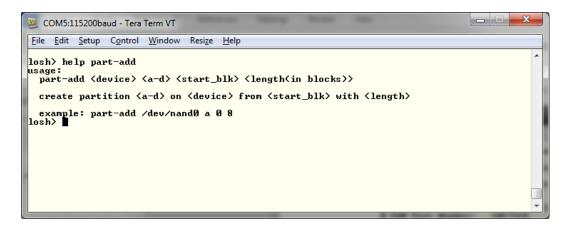
The device we're adding the partition to is *nand0*. Since LogicLoader resides in the first partition, this is the second partition and it will be partition b. The partition will start at block 18 and go to block 2048. So, type part-add /dev/nand0 b 18 2030.
