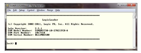
Note the string LoLo Version: 2.5.1 in the image above. This tells us that the development kit is running version 2.5.1 of the LogicLoader software. This version of LogicLoader also provides the SOM model number, part number and serial number. This allows you to send one screenshot to Technical Support and have all of the information in one place.
