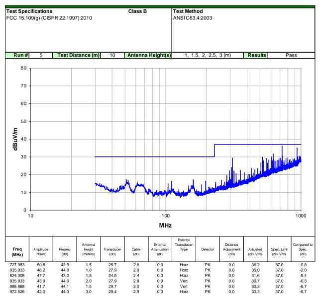
Figure 3.1: PXA270-11 Card Engine Scan (CENGPXA270-520-11-504HCR)
