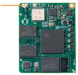
Figure 4.2: Antenna Connector Location on AM3517 SOM-M2
